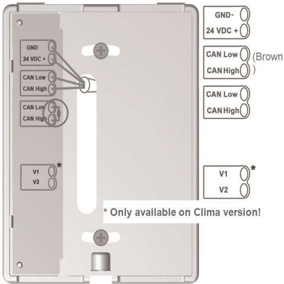
Open the terminals with the accompanying operating tool and make the electrical connection as described.
