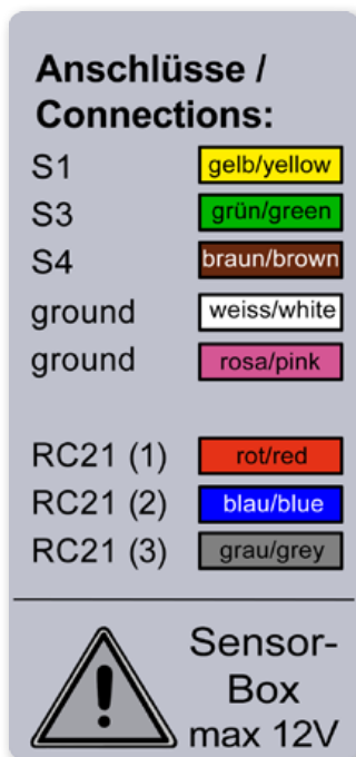
Picture 1: Connection of the sensors to the sensor box
