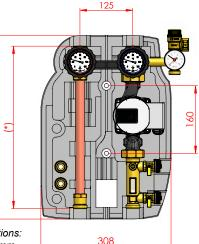
(\*) Distance of threaded connections: 22 mm compression end: 405 mm 3/4"M and 1"M: 385 mm
