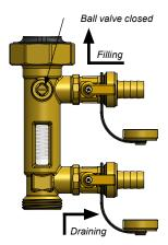
3. Remove the plugs from the side valves and connect the hose unions, by connecting them to the filling device of the system;
