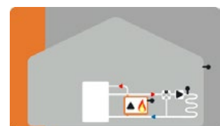
Combined storage or buffer storage with mixed heating circuit with additional function burner and boiler pump.
